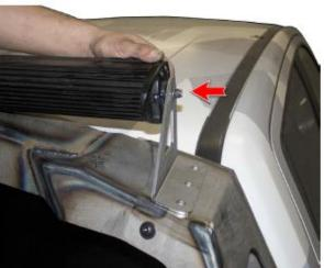
8. Install the supplied 3/8" Bolts (x4), 3/8" Washers (x8), and 3/8" Lock Nuts (x4) into the other side of the center rail. (Fig E) One washer under head of bolt, one washer under nut.
