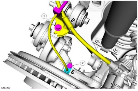
14.3 Install the lower arm vertical link. Position the lower arm vertical link and install the 2 lower arm vertical link bolts.
