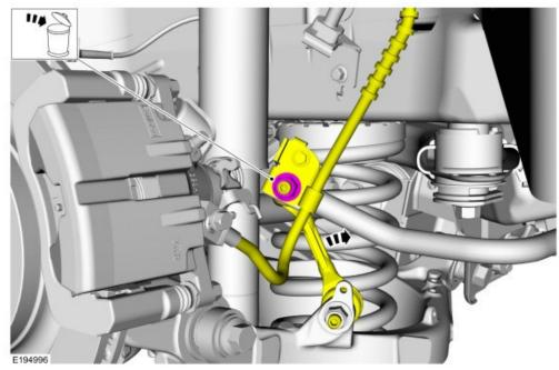
17.2 Remove the 4 stabilizer bar bracket bolts and remove the stabilizer bar.
