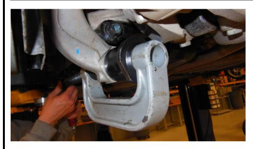
9.2 With the old bushing removed, set up your ball joint press with new bearing to press in knuckle.
