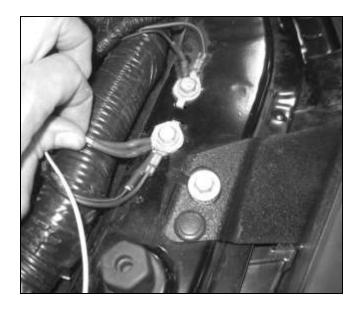
Route the single wire with two electrical connectors along the factory engine harness to the rear
