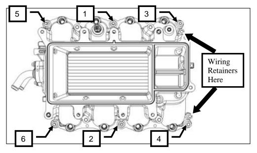
3. Lube the fuel injector o-rings with assembly lube. Install the fuel rail and injectors into the intake manifold using the take off bolts. Be sure each injector is properly seated into the intake manifold. Tighten the bolt pattern in two stages. Stage 1; torque bolts to 10 Nm. Stage 2; tighten bolts an additional 90 degrees.
