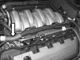
a) Install one length of protective sleeve onto the passenger side heater hose. Slide it over the quick connect fitting and along the heater hose. Apply electrical tape over either end of the protective sleeve to secure its position on the hose.
