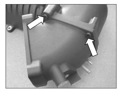
7. The supercharger is shipped without oil in the front gear case. A bottle of supercharger oil has been included in your supercharger kit. Place the supercharger assembly on a flat and level surface and fill the front case with oil per the following instructions:
