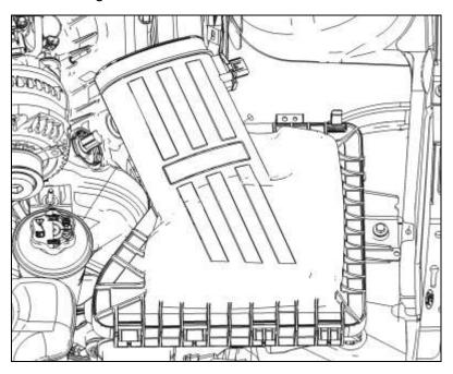
2. Insert the Vacuum Fitting (383004-S) and the ½" Vacuum Cap (CS515) from Hardware Kit A into the Clean Air Tube (1312-9R504) in the orientation shown.
