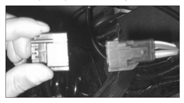
4. Populate the new connector such that the yellow with violet wire is in position 1, the blue with green wire is in position 2, the brown wire is in position 3, the blue with orange wire is in position 4, the yellow wire is in position 5 and the green with violet wire is in position 6. Install the red plastic lock into the connector to secure the wires in place.
