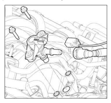
2. Install the valve into the new Throttle Body Spacer using (2) M6 x 1.0 x 35.5 mm bolts (N808429). Torque bolts to 10 Nm.
