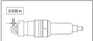
2. Install the re-gapped spark plugs. Torque to 14 Nm (124 lb-in). Install the ignition coil on plugs. Apply a small amount of dielectric grease to the inside of the coil on plug boots before attaching to the spark plugs. Torque the bolts to 6 Nm (53 lb-in). Re-install the coil on plug covers.
