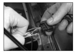
3. Perform a visual inspection of the newly pinned connector to ensure that wire colors match on both sides of the harness. Re-install the pin locking device on the front face of the connector.
