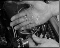
2. Insert the pins from the factory connector into the female connector provided on the end of the MAF Extension Harness (131112B579W). The following color wires go into the following positions on the clip: Violet with Grey – position #2, Grey with Yellow – position #3, Blue with White – position #4, Yellow with Violet – position #5. NOTE- Positions 1 & 6 are not used.
