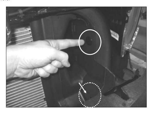
2 - Cut the rubber edge of the side shield in three (3) places as shown.
