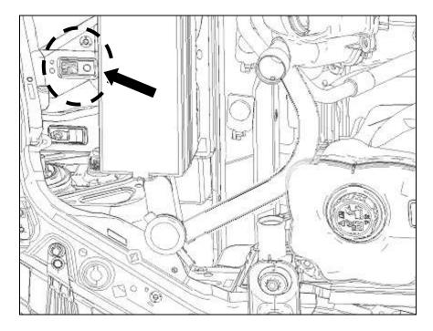
2. Install the relay from the Intercooler Pump Wiring Harness (13118W501) onto the stud. Install the fuse on top of the relay onto the same stud. Use (1) M6 nut (W520412) from the Intercooler Hardware Kit (13116066FRTHKE) to secure the relay and fuse to the stud. Torque the nut to 10 Nm. Reinstall the wiring harness from previous step to the stud for proper retention.
