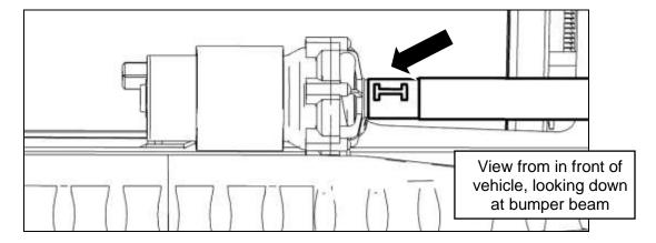
11. Route the remainder of the Intercooler Pump Wiring Harness next to the headlight and radiator and through the hole in the RH Radiator Side Shield. Connect the wiring harness to the pump and secure the harness to the bracket by pushing the push pins on the harness into the holes in the mounting bracket.
