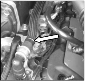
6. Install the 3/8" Engine Bottle Degas Hose (13118276) from the engine degas bottle to the fitting on the driver side cylinder head. Secure with the constant tension clamps removed from the factory hose. Ensure both 3/4" intercooler hoses, the degas hose and all clamps and wiring have been installed to provide maximum clearance to the supercharger belt.
