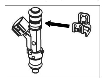
2. Apply assembly lube to the injector O-rings and install the injectors into the new Fuel Rail (13119F792). NOTE: Verify that the anti-rotation clips are properly aligned and fully engaged into the fuel rail injector cups.
