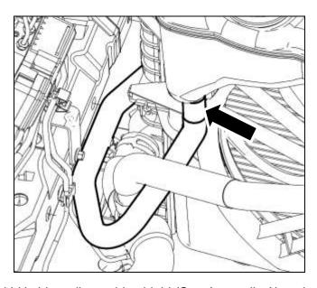
2. Install the modified LH side radiator side shield (See Appendix A) and route the Intercooler Pump Inlet Hose (installed in the previous step) through the new hole in the shield and secure the shield to the chassis using the take off push pins.
