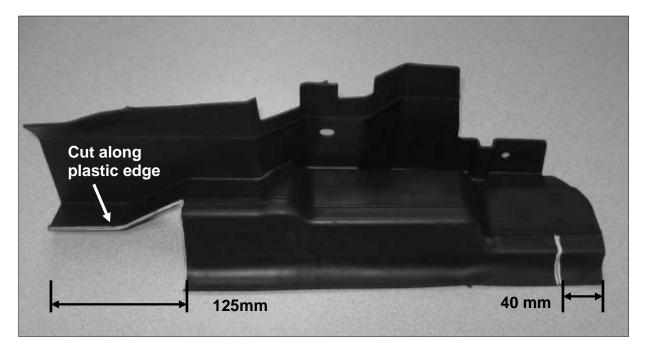
7 - Re-install the RH radiator side shield using the take off push pins.
