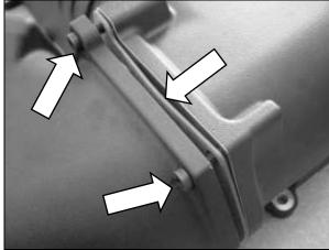
14. Connect the bypass actuator hose from the ½" port on the throttle body spacer to the port on the bypass actuator. Ensure that the rubber 90° elbows are fully installed on both ends.
