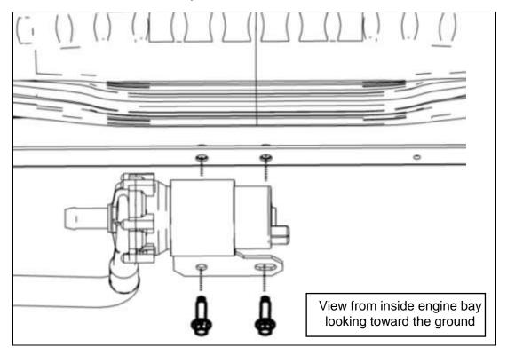
9. Connect the Intercooler Pump to LTR hose to LTR inlet port using (1) 3/4" constant tension clamp. Orient the clamp so the "I" on the hose is in the center of the clamp tangs.
