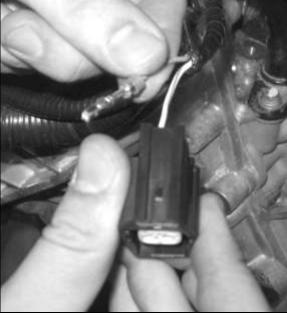
Connect the Canister Purge Valve Extension harness to the newly installed connector. The wire
