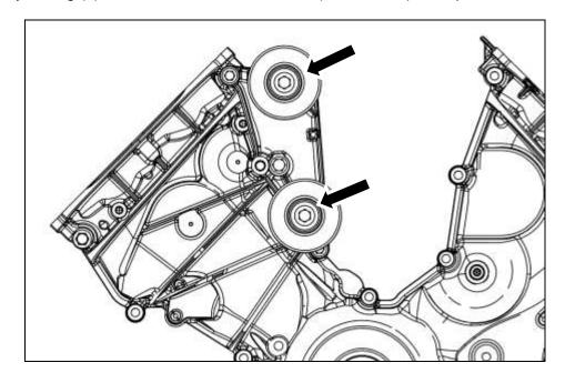
Loosely install the FEAD Tensioner Bracket Assembly (13118B603) onto the front cover using (2) M8 x 1.25 x 123mm (R18020055) bolts, leaving atleast a 10mm gap between the two new FEAD brackets.
