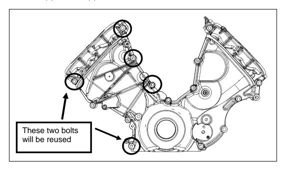
2. Install the Upper FEAD Bracket (13118B653U) using (2) M8 x 1.25 x 57mm bolts that were removed in the previous step and (2) M8 x 1.25 x 84mm bolts (W704752) from Hardware Kit C. Torque bolts to 25 Nm.
