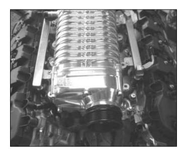
9. Install the (9) M8 x 1.25 x 30 fasteners provided in the kit into holes 1, 2, 3, 5, 6, 7, 8, 9 and 10.
