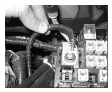
4. Route the other bundle of wires coming from the relay around the front of the fuse box along the factory forward lamp harness. Remove (1) bolt securing the factory ground wires to the chassis behind the headlight. Replace the bolt to secure the factory grounds including the grounding eyelet from with the intercooler pump harness.
