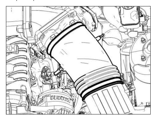
4. Install the PCV Fresh Air Inlet tube (13116758) by connecting the 90 deg fitting to the driver side cam cover and angled fitting to the PCV fitting in the clean air tube.
