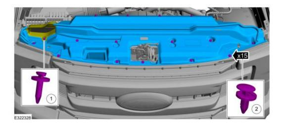
2. Remove the retainers along the top of the panel. *Torque*: 36 lb.in (4.1 Nm)
