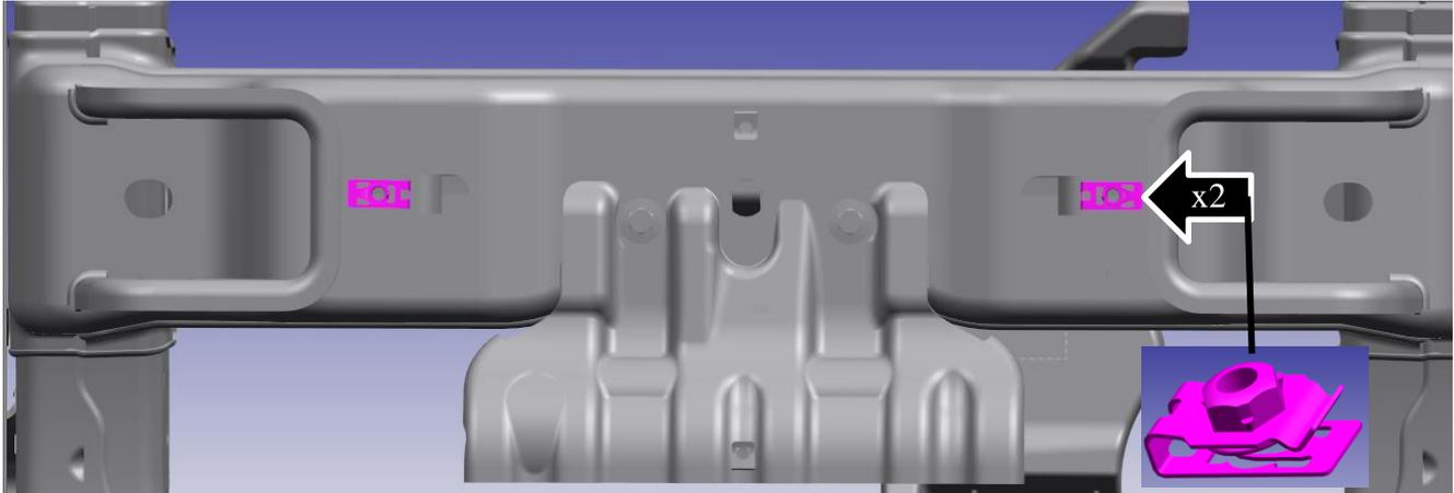
4. Attach the skid plate brackets to the frame using the bolts and washers (M10x35).
