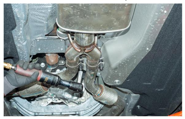
STEP 5: Using a muffler stand or additional person, remove the factory system from vehicle.
