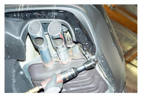
STEP 3: Remove the under-axle hanger brackets from the frame, retain the hardware.
