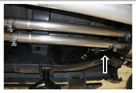
Install the Mid Pipes. One Mid Pipe will Have an Exhaust Hanger, one will not. The one WITH the Hanger goes to the outside of the Vehicle. (see Arrow). **Do not tighten the Clamps at this time.**
