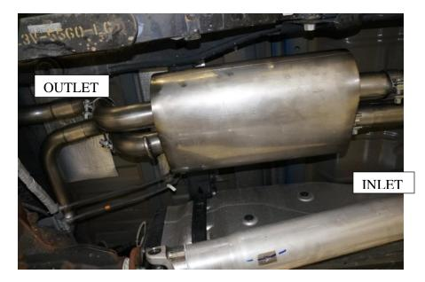
Slide another Two (2) Clamps over the Muffler Inlets. Position the Clamp with the Nut facing down and to the outside of the Vehicle. With the help of an Assistant, Install the Muffler by putting the Muffler Outlets OVER the Rear Axle first. Then Align the Muffler Inlets with the Mid Pipes and slide the Muffler Forward. Install the Muffler Rear Hanger with the original Bolt.
