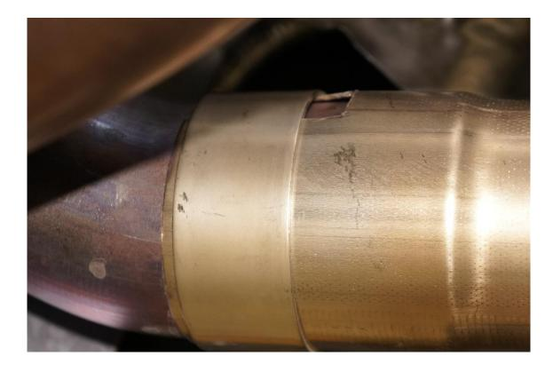
**IMPORTANT NOTE!!!!** Pay VERY close attention to the Inlet Tube Orientation Keyway. The above Picture shows that the Band Clamp needs to be slid back in order to cover this area. Also important is to be sure the Pipe Clamp Nut and Bolt are never over a relief cut. Please take extra time to ensure these areas are well secured.
