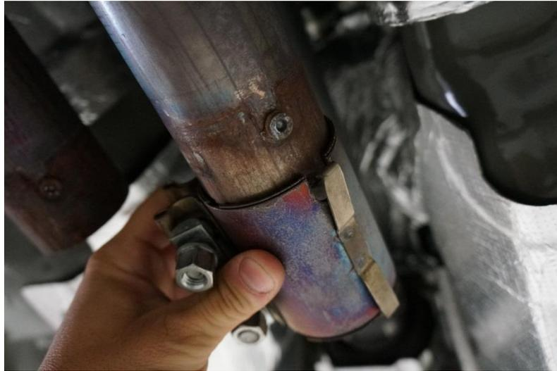
**Step 7:** Allowing exhaust to hang down, remove rear mufflers from hangers by moving the exhaust system towards front of vehicle.
