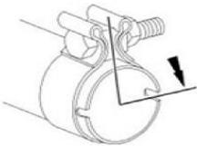
**To tighten the exhaust clamp.**
