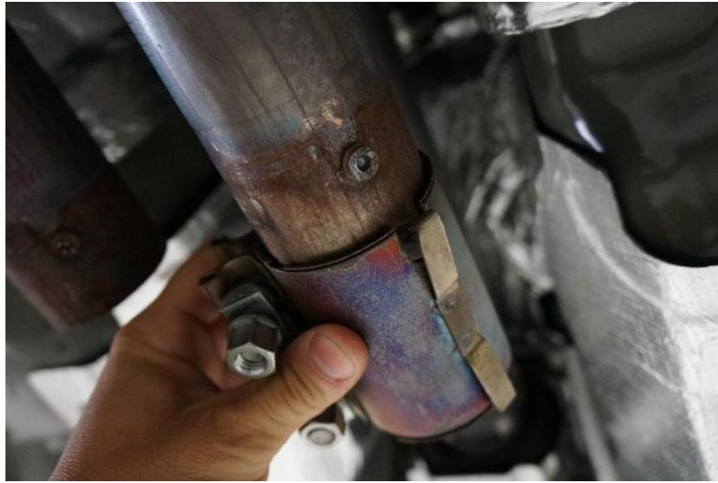
**Step 2: Install new front muffler (or x-pipe) onto clamps. Snug but do not tighten.**
