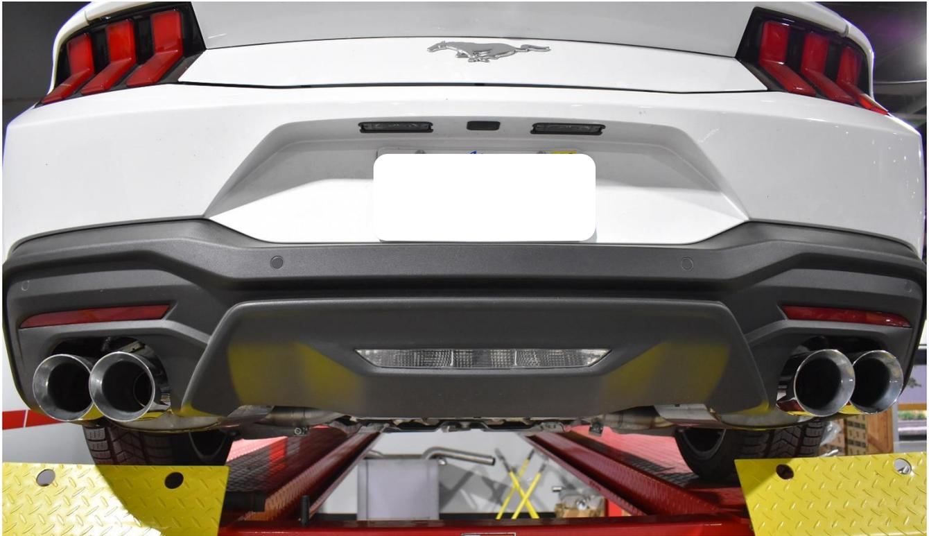
**STEP 8: Start vehicle and check for any leaks. If any leaks are found, determine cause (such as loose or incorrectly positioned clamp) and repair as necessary.**
