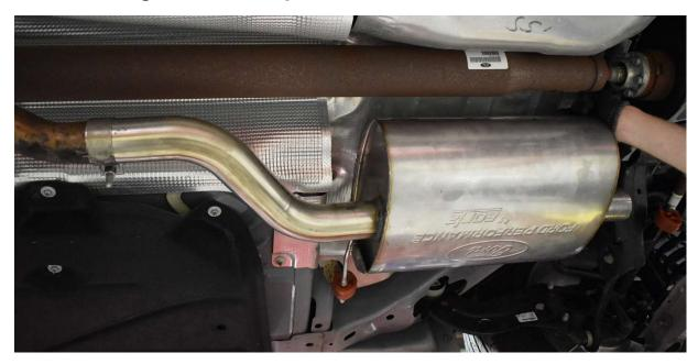
STEP 2: Slide a clamp over the expanded inlet of the underaxle pipe. Slide onto the muffler outlet, and push the hanger into the rubber isolator.
