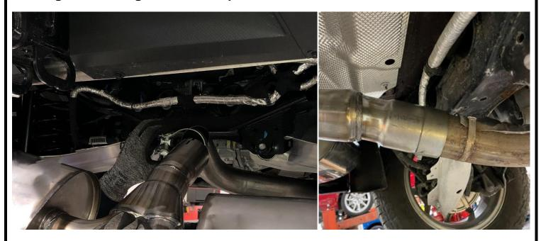
Step 3: Place (2) hangers into the rubber isolators.
