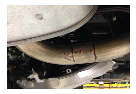
Drivers side muffler (Cut line is the start of the bend going into the muffler)
