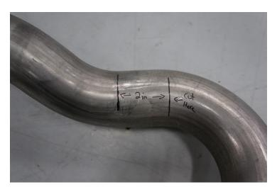
STEP 4: After cutting is completed remove muffler from rear hanger, deburr intermediate pipe. For vehicles with valves, disconnect the valves at the rear mufflers (LH and RH). Pull the pin holding the connector in, slide it out of the valve actuator assy.
