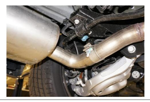
Step 3: Install passenger hand muffler into rear hanger slide clamp onto muffler pipe, slide muffler onto the pipe that you just cut. Position tips in cutout and torque clamp to 48Nm (35 lb-ft).
