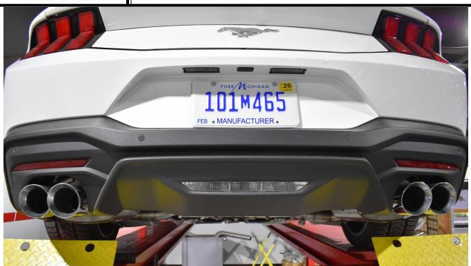
STEP 9: Lower vehicle. Start vehicle and check for any leaks. If any leaks are found, determine cause (such as loose or incorrectly positioned clamp) and repair as necessary.
