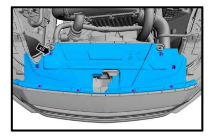
16. Remove the (7x) fasteners from fascia. Carefully pull the fascia forward.
