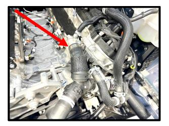
63. Using 10mm socket, remove the (3x) factory fasteners from the timing chain to head cover and (1x) from water pump (for new idler plate), this includes the factory ground wire/eyelet.
