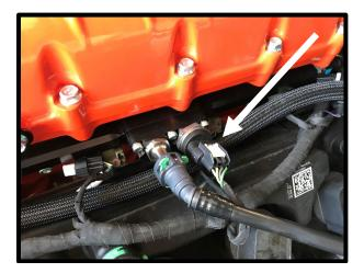
106. Install (1x) #906 oring to the supplied (1x) -6 ORB to 9.89mm quick connect fitting. Install fitting to the **LH** side port using an 11/16" socket.
