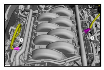
40. Remove the (4x) nuts from the top of the intake manifold, remove heater hose supports.
