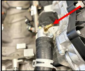
56. Trim the reservoir vent line right at the ENG printing on hose. Reinstall stock hose to new fitting. Secure with supplied #4 clamp.
