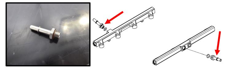
76. Apply light amount of grease to -6 ORB plugs, install the supplied (2x) -6 ORB plugs to front fuel rail ports.
