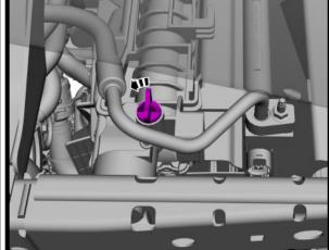
32. Disconnect the MAF sensor, MAF sensor retainer and remove make up air hose from air tube.
