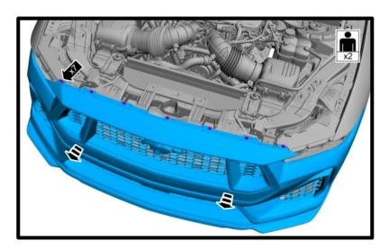
153. Install the radiator sight shield, secure using the (8x) push pins.
