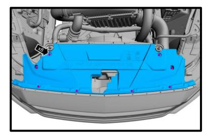
154. On both sides, install front bumper cover to fender with original push-pin and the bolts. Torque to 44 lb-in.
