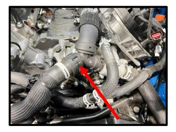
55. Transfer stock oring from stock water neck to new water neck. Apply pipe sealant to threads of 1/8" NPT to 5/16" 45 Deg fitting. Install fitting to water neck, rotate so it ends facing directly towards driver side. Install water neck to motor using stock fasteners (10mm socket), torque to 89 lbs-in.
