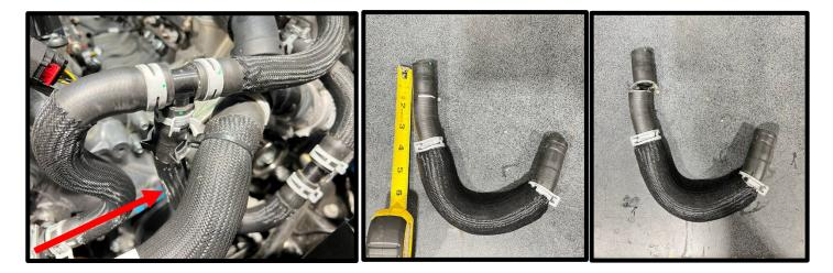
61. **(Auto Transmission)** Connect U shape hose back to stock tees, install/position to **FRONT** side of radiator hose (this stops it from getting to water pump pulley. Rotate the factory hose retainer and connect to this hose to secure in place.
