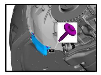
7. **(GT ONLY)** On both sides, remove the (4x) push pins and position aside the front fender splash shield.
