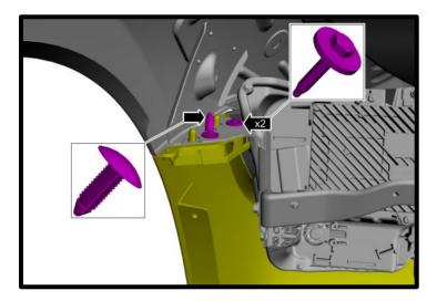
15. Remove the radiator sight shield by removing the (8x) push pins. Use a flat head screwdriver to pry the center head up. These will all be reused.
