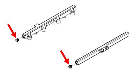
77. Install supplied (2x) #2-906 orings to (2x) -6 ORB to 9.49mm short fittings. Install the (2x) fittings into rear side of fuel rails. Apply light amount of grease to oring for ease of installation. Using a ¾" wrench (or ¾" deep socket) on both the front and rear fittings, tighten both.
