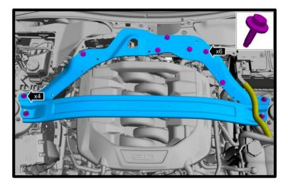
30. Lift and remove cover from the engine.
