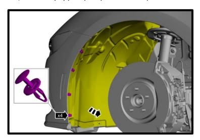
162. On both sides, install the (4x) fasteners to body side front shield, torque to 18 lb-in.
