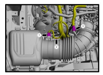
33. Loosen the hose clamp from throttle body using nut driver. Remove the air cleaner bolt. Detach the air cleaner from grommets and remove the air cleaner.
