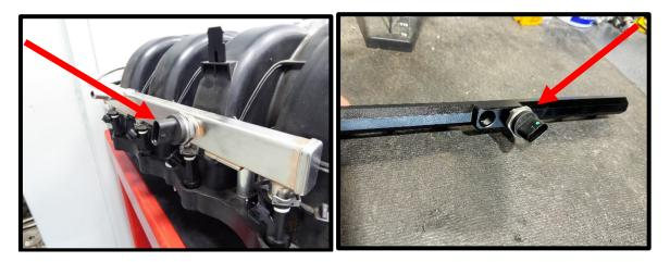
75. Install supplied (2x) #2-906 Viton oring to (2x) 45mm long 9.49mm fuel fittings. Apply light amount of grease to oring for ease of installation and install fitting. Install fittings, one per rail.
