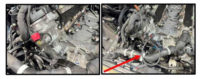
85. Remove plastic harness retainers from loom at the back of the engine.
