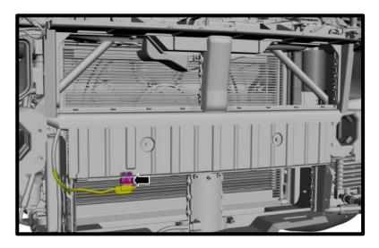
152. Install the (7x) fasteners from fascia.
