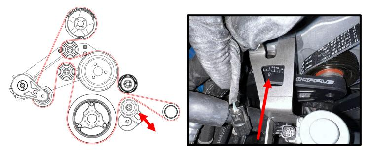
97. With belt holding the SC pulley in position, torque the supercharger (5x) 6mm x 15mm SHCS bolts to 130 lbs-in using a 5mm allen socket. Do not use Loctite on threads, it is not required.
