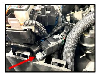
129. Locate stock ground wire stud, located on RH side of vehicle, next to strut tower brace using an 8mm socket. Install intercooler relay harness ground eyelet (black wire) along with factory ground wire. Reinstall bolt using an 8mm socket.
