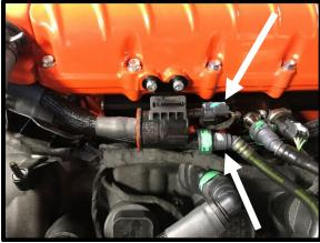
108. Install supplied 3/8" ID x 5 ½" with 55deg quick connect fitting hose (#5000030) to the EECPV barb fitting and **LH** quick connect fitting on SC inlet. Push until it clicks and locks into place.
