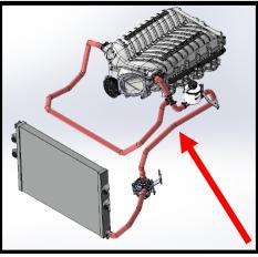
124. Install hose #3103406 from **LH forward** most IC fitting (outlet). Secure hose to IC fitting with #16 Black worm clamp. Install TEE fitting with TEE facing forward. Install supplied 90deg hose #3103158 to end of TEE and secure to front most IC filler reservoir fitting (inlet). Secure 90deg hose to tee and reservoir with #16 Black clamps.
