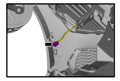
13. Disconnect the front bumper cover electrical connector.
