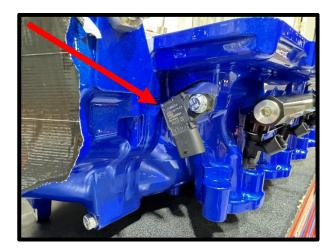
84. Install supplied electronic throttle pigtail to the factory **RH/PASSENGER SIDE** electrical connector. Push until it locks in place, then lock the safety lock. Route to **LH** side of vehicle for later connection to throttle body. **TIP:** When pressing together, hold the wires and connector to ensure the wires cannot come loose during connection.
