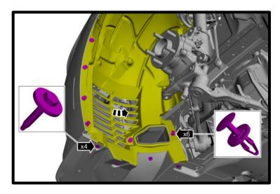
9. **(GT ONLY)** Remove the (12x) fasteners from the front chin splitter.
