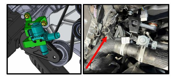
72. Install supplied (2x) smooth aluminum idler pulleys (**#3102717**) to the idler plate. Secure using the (2x) step washer through front of bearing and (2x) ½"-13 x 1 ¾" SHCS (with light amount of anti-seize on threads) bolts. Torque to 30 lbs-ft. using a 3/8" allen socket.
