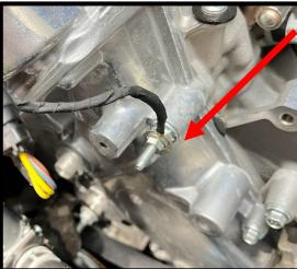
64. Using 10mm socket, remove the stock fastener (1x) from the top of the RH timing chain cover. Relocate stud with ground wire to the top timing chain cover location. Torque to 22 lbs-ft.
