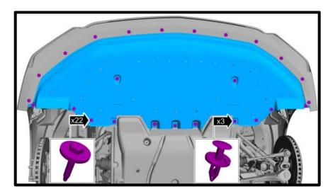
11. (DARK HORSE) Remove the (24x) fasteners and (3x) push pins from underbody shield.
