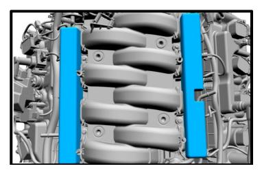
42. Loosen the (4x) bolts holding the fuel rails down, these go through to the cylinder head (10mm socket). Fuel rail does not need to be removed.
