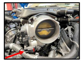
137. Install supplied (1x) 3/8" to 15.82mm hose adapter to the inlet tube 3/8" boss.
