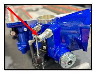
110. Install supplied 1/2" ID x 9" hose (#3103159) to the passenger side valve cover. Connect other end to supercharger inlet quick connect fitting. Push until it clicks and locks into place.
