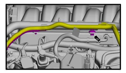
38. Detach the heater hose retainer. Remove the heater hose from both driver and passenger side of block by pulling locking tab back and pulling away. Position the heater hoses aside.
