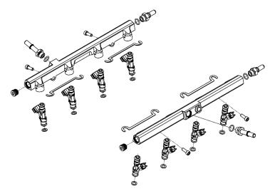
79. Apply generous amount of grease to injector orings for ease of installation. Install supplied fuel injectors, rails and lock bracket to intake manifold, secure with the (4x) 6mm x 16mm SHCS using a 5mm allen socket. Use **Blue Loctite** #243 on the threads of each bolt. Torque to 90 lbs-in.
