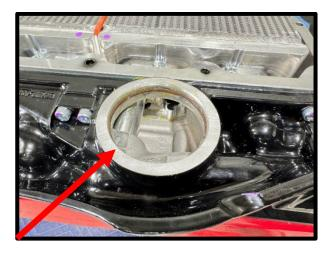
101. Apply generous amount of grease to the (1x) #2-230 Viton bypass oring. Install the supercharger lid to the supercharger housing by carefully placing the bypass down. Secure the SC lid using the (17x) 6mm x 30mm HHFCS and (3x) 6mm x 70mm HHFCS (*marked green*) using the following pattern. Torque to 90 lbs-in using an 8mm socket.
