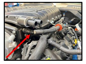
109. Install (1x) supplied #906 oring to the (1x) -6 ORB to 15.82mm quick connect fitting. Install fitting to **RH** side on the inlet using a 7/8" socket.
