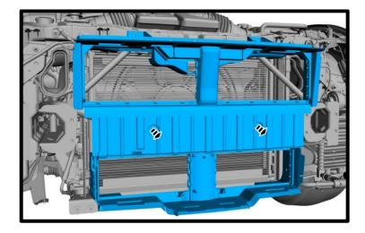
23. (Vehicles equipped with active shutter grilles) Release the tabs and remove upper linkage.
