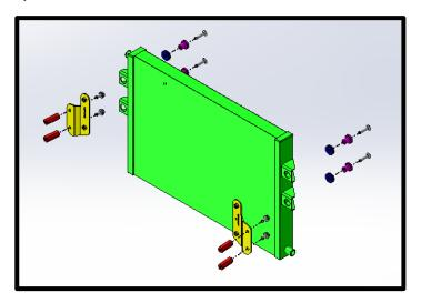
114. Slide the LTR assembly up from the bottom. Connect the LTR brackets to the coupling nuts using the supplied (4x) 8mm x 16mm hex headed flanged bolt (12mm ratchet wrench).
