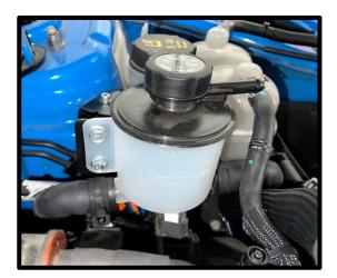
117. Mount IC pump bracket to the LH inner frame rail, using (1x) 8mm x 16mm HHFCS bolt.
