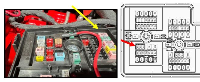
131. Use small set of cutters or file, make a small notch in fuse box cover lid and fuse box to allow wire to fit. use small file to clean up and round edges
