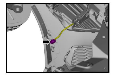
157. **(GT ONLY)** Install the (22x) fasteners and (3x) push pins, torque to 18 lb-in.
