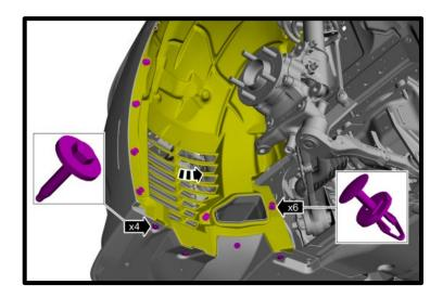
161. (GT ONLY) On both sides, install the (4x) push pins tp front fender splash shield.
