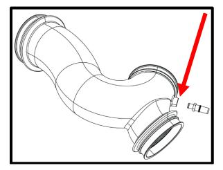
138. Install factory MAF sensors to the new MAF housings using supplied (4x) 4mm x 10mm SHCS. Torque to 17 lbs-in. \*\*DO NOT USE STOCK BOLTS\*\*. \*NOTE: Verify arrow position for airflow direction.
