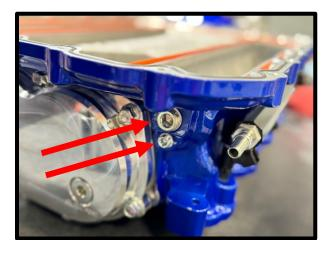
74. Using 27mm socket, remove the fuel PSI sensor from the factory fuel rail. Using 27mm socket, remove fuel PSI sensor from factory fuel rail. Install factory fuel PSI sensor to the fuel rail using a 27mm socket. Torque to 53 lbs-in, then an additional 25-degree rotation. **NOTE: Never use sealant on these threads.**
