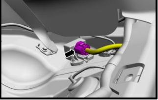
4. Locate the battery. Remove the plastic cover, (1) retaining clip and (3) retaining nuts for battery access. With an 8mm wrench disconnect both (-) battery cables from battery. Make sure the cables are far enough away from the battery that it does not accidentally touch the battery and make connection during installation.
