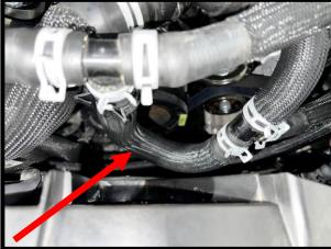
62. Using 5/16" nut driver, secure hose using supplied #24 hose clamp. Rotate the clamp at water neck towards the driver side for future clearance of the SC.
