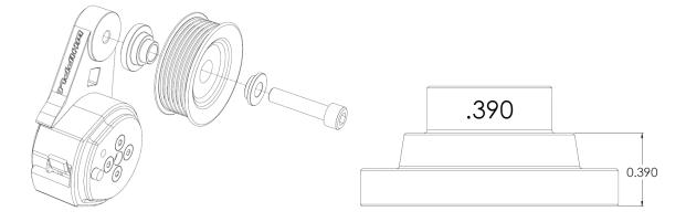
68. Carefully bend the factory AC line down and towards passenger side. Install spring loaded tensioner to plate to check clearance. You should have a minimum of 3/8" of clearance from the tensioner to the AC line.
