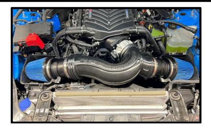
142. Install supplied ½" x 13 ¼" make up air hose to the LH valve cover. Push until it clicks and locks into place. Install other end to air inlet tube fitting previously installed.
