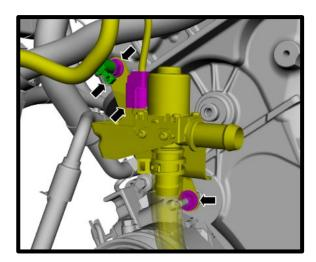
59. Remove stud from engine timing cover, this will not be reused.
