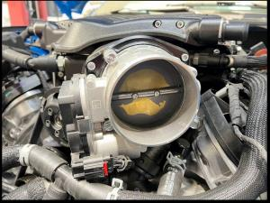
136. Connect previously installed throttle extension pigtail to the throttle body electrical connector. Secure wiring using zip-tie. **NOTE: Failure to secure wire may result in the wire catching the belt system!**
