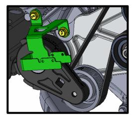
71. **(Auto Transmission)** Mount trans cooler solenoid to the supplied bracket using (4x) stock fasteners. Connect extension harness to stock connectors.
