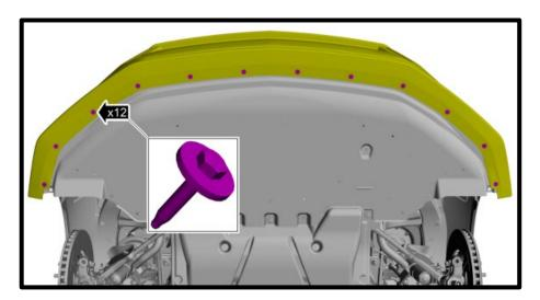
10. **(GT ONLY)** Remove the (22x) fasteners and (3x) push pin from the underbody shield. Remove shield from vehicle.
