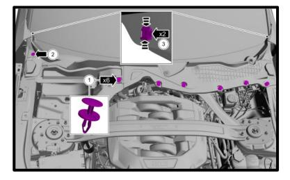
147. Install the (6x) bolts and position active grille shutter **SHELL ONLY (shutter grilles are NOT reused)**. Torque to 71 lb-in.
