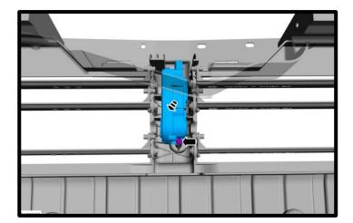
26. Remove the (6x) push pins (1), (2x) retainers (2) and depress and remove the clips (3) (2x).
