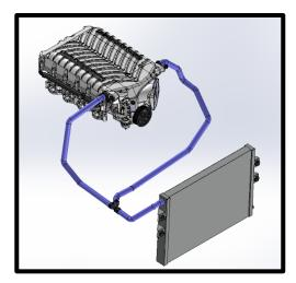
123. Install hose #3103405 from rearmost IC filler reservoir fitting to the top IC pump fitting (inlet). Use supplied #16 pinch clamps to secure hose.
