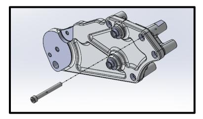
93. Torque (10x) 6mm HHFCS manifold bolts in the following pattern using a 10mm socket. First pass: 88 lbs-in. Second pass: 106 lb-in. **NOTE:** For bolt #10, a ¼" socket with 4"-6" extension, 10mm wobble is the best possible tool to get into this tight area.
