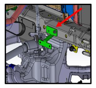
118. Mount IC pump clamp to the pump bracket using (2x) 6mm x 8mm HHFCS bolts. Install pump to clamp, pump inlet should be facing the front of the vehicle. Leave loose until IC hoses are installed.
