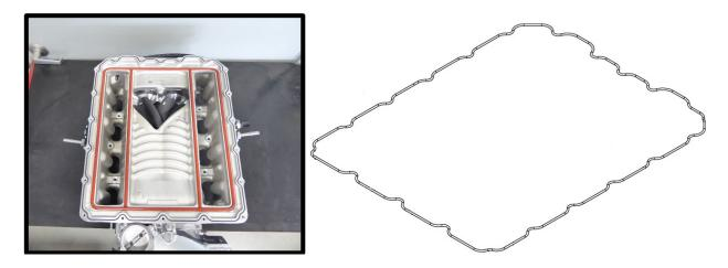
100. Install (1x) #2-230 internal bypass oring to the lid bypass passage. Use generous amount of grease to secure oring in place and help with installation.
