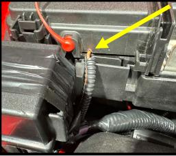
133. Using a 10mm socket, remove the 12V (+) power stud nut from the far post. Install the IC pump relay power eyelet (red wire) to the 12V stud. Use a 10mm socket to secure stock and IC power wire.
