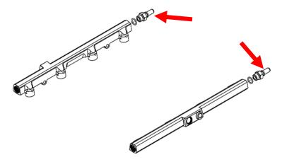
78. Install fuel injectors to the fuel rail, apply generous amount of grease to oring for easy installation. Install supplied fuel injector position lock bracket to clock the supplied fuel injectors into proper position. While installing lock bracket, secure fuel injectors so it doesn't add pressure to injector body. **CAUTION:** *Failure to clock the injector correctly can cause severe running issues.*
