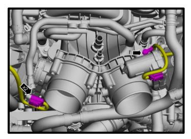
37. If equipped, detach the wiring harness retainers.
