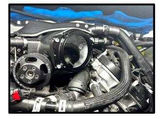
135. Install supplied (1x) #2-045 V75BR oring to TB adapter. Install the stock throttle body using the (4x) 6mm x 35mm HHFCS bolts using a 10mm socket.
