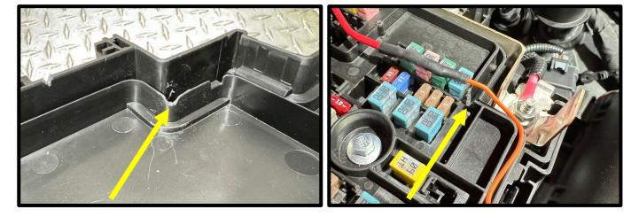
132. From fuse tap, route to slot you previously made. Route to stock slot at the front of fuse box. Add small relief in lid for wire as it comes out of the box. use small file to clean up and round edges. Test fit lid and ensure it does not interfere with this wire. Failure to route properly will lead to IC pump operation failure, resulting in poor performance.
