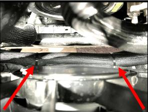
126. Secure supplied 3/8" 90deg hose to IC filler reservoir top barb using #4 hose clamp. Route down and secure hose to 3/4" IC pump feed hose using zip tie. Route down away from engine.
