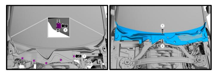
28. **(LHD ONLY)** If equipped, remove the strut tower brace by detaching the battery wire retainer. Remove the (4x) nuts and (5x) bolts. Reinstall factory nuts (4) and torque to 41 lbs-ft.
