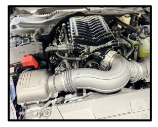
144. Reinstall the K-Brace over the studs and into position on the vehicle. Install the (2x) nuts on the studs and torque to 25 Nm using a 15mm socket. Install the (5x) mounting bolts and torque to 25 Nm using a 13mm socket. Reinstall the (7x) pushpin retainers on the cowl trim panel.
