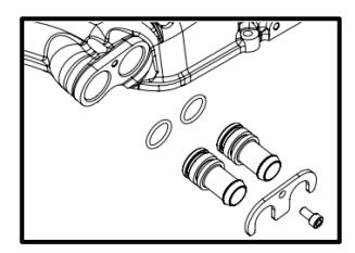
103. Connect factory passenger side rail fitting to the DI pump factory hose, press until it clicks and locks in place. NOTE: THIS FUEL LINE HAS A CHECK VALVE, DO NOT FLIP ORIENTATION FROM STOCK DIRECTION. THE 90-DEG END ALWAYS CONNECTS TO FUEL FEED SUPPLY FROM FUEL RAIL! 30-DEGREE ALWAYS CONNECTS TO PUMP!
