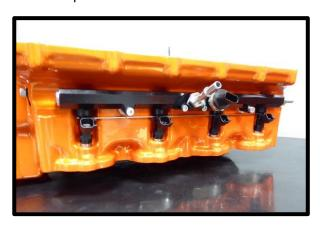
80. Install supplied 3/8" fuel cross over line around back of the supercharger by pressing until they click and lock in place. \*NOTE: The 90deg end goes to LH side.
