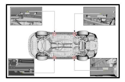
6. On both sides, remove the (4x) fasteners from body side front shield.
