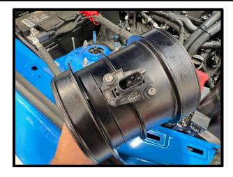
139. Install supplied filters to MAF housing, secure using supplied filter clamp. Install the MAF housings into the Y tube (for ease of installation), pre-install #80 hose clamp to Y tube, leave loose until later.
