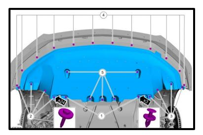
159. **(GT ONLY)** Install the (12x) fasteners to front chin splitter, torque to 18 lb-in.
