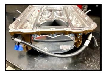
81. Install supplied ¼" ID bypass actuator to bypass nipple and ¼" 90deg nipple on SC inlet. **CAUTION:** Do not open/close bypass actuator by hand. This may damage actuator internally. It only moves properly with equal vacuum/boost at the actuator reference port.
