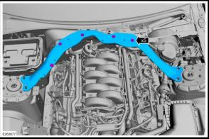
145. Install the (5x) push pins (1) and depress the (2x) clips (2).
