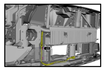
149. If equipped, reconnect the CCM wiring connector.
