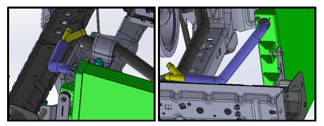
121. Install hose #3103408 from offset Y straight to **RH rear** most IC fitting (inlet). Use supplied #16 silver worm clamp to secure hose to Y and #16 Black clamp to IC fitting. **NOTE:** Routing IC hose incorrectly can result in poor performance and potential damage!
