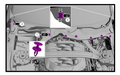
27. Remove the (5x) push pins (1) and depress the (2x) clips (2). Lift and then pull cowl panel grille out and remove.
