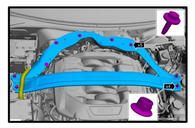
29. **(RHD ONLY)** If equipped, remove the strut tower brace by detaching the battery wire retainer. Remove the (4x) nuts and (6x) bolts. Reinstall factory nuts (4) and torque to 41 lbs-ft.
