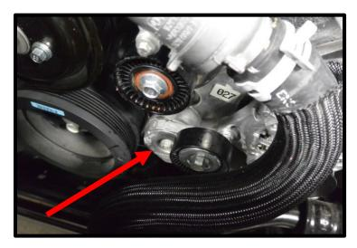
50. Remove the water pump pulley using a 10mm socket (this will be reused).
