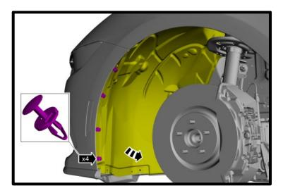
8. (**DARK HORSE**) On both sides, remove the (4x) fasteners and (6x) push pins from front fender splash shield.
