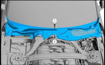
146. Install the (6x) push pins (1), (2x) retainers (2) and the clips (3) (2x).
