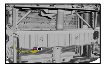
18. Temporarily remove the retainers (4x per side) from air ducts and remove ducts.
