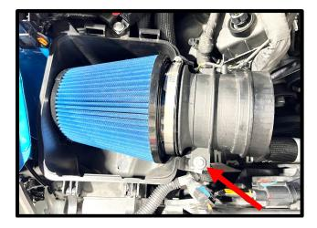
141. Install the inlet tube to the MAFs and throttle body. Secure using the supplied clamps, (2x) #80 on MAF side and (1x) #64 to throttle body. Reconnect MAF connectors to MAF sensors.
