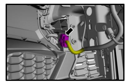
14. On both sides, remove the front bumper cover to fender push-pin and the bolts.
