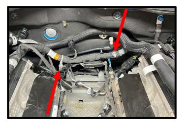
86. Install supplied TMAP pigtail to stock connector at rear of engine. Route to **LH** side of vehicle for later installation to supplied 3-Bar TMAP sensor.
