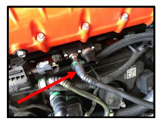
105. Connect the factory fuel PSI sensor connector to sensor, press safety lock until it clicks and locks in place.
