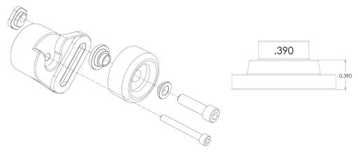
67. Assemble spring-loaded tensioner by mounting supplied spacer with female register to tensioner. Install grooved idler pulley (**#36326**) to tensioner and (**.390**") step spacer. Use supplied step washer to front face of pulley bearing and (1x) 10mm x 40mm SHCS (**10-Rib uses 10mm x 60mm SHCS**) bolt. Use light amount of anti-seize on threads. Torque to 18 lbs-ft. **NOTE:** Verify you're using the proper spacer as shown.
