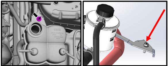
116. Mount IC reservoir to bracket using (2x) 6mm x 12mm HHFCS.
