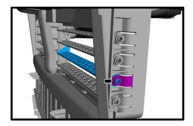
25. **(Vehicles equipped with active shutter grilles)** Remove the bolt and the active grille shutter actuator. **NOTE:** These are no longer used.
