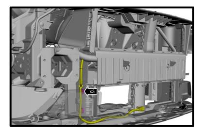
20. Remove the (6x) bolts and position active grille shutter forward.
