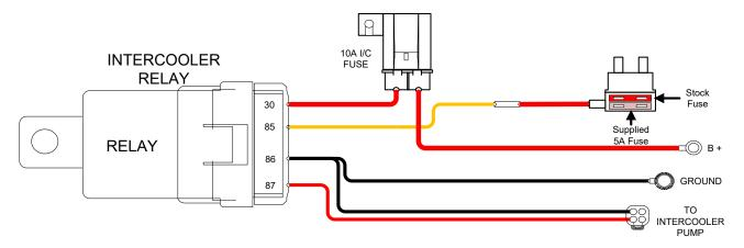
128. Mount relay and fuse holder to the factory airbox stock fastener, secure with zip-tie. Route 2-wire connector down, below radiator, along sway bar to the LH side of the vehicle. Connect to IC pump. Secure harness using zip-ties along bottom of vehicle.
