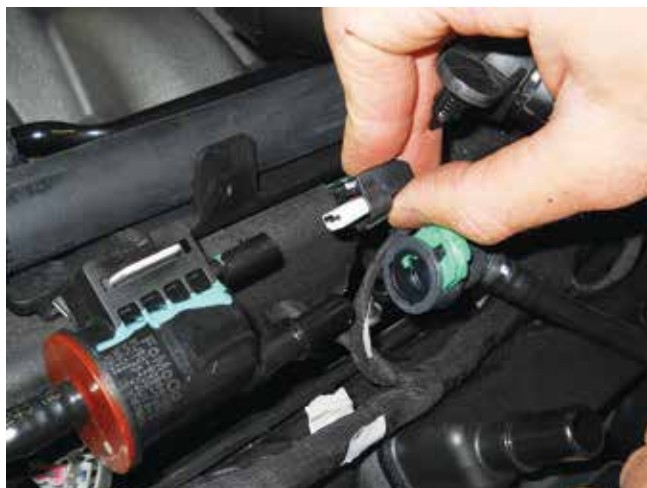
EECPV electrical connector
