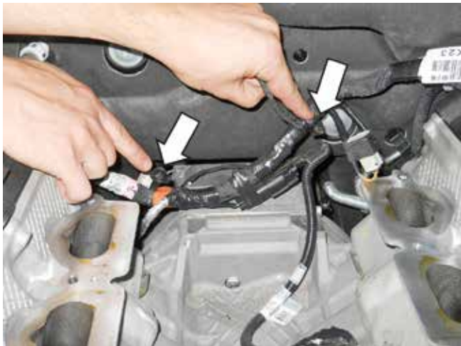
Pin retainers on harness
