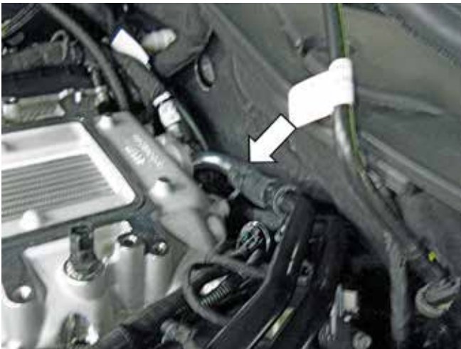
11. Connect the ACT sensor to the ACT harness (1318-12B579W).
