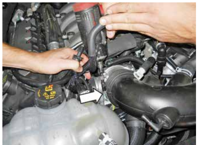
Clamp at throttle body
