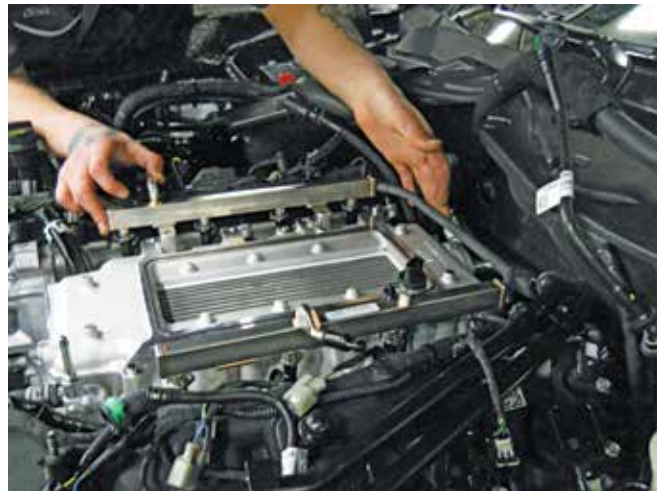
13. Install the M6x1.0x20 fuel rail-to-intake manifold bolt (BM6X20HF-S437) (short) at position 2 and M6x1.0x45 fuel rail-to-cylinder head bolt (161817) (long) at position 4 . 4. Tighten the bolts in two stages in the sequence shown. Install original takeout bolt in position 5 Stage 1: Torque the bolts to 10 Nm. Stage 2: Tighten the bolts an additional 45 degrees.
