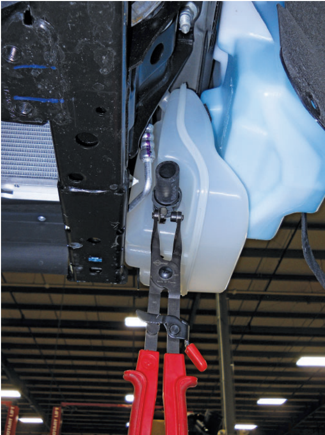
2. Install the intercooler pump (1318-8501, found in 1318-KIT4) onto the bottle hose and slide the clamp over the water pump.
