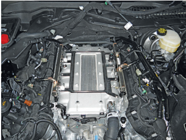
14. Connect the eight (8) fuel injector electrical connectors.
