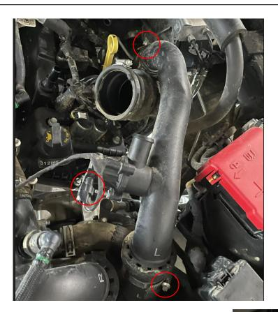
For tube removal, start with removing the upper tube with bypass valve, loosening 2 hose clamps and disconnecting the bypass valve.
