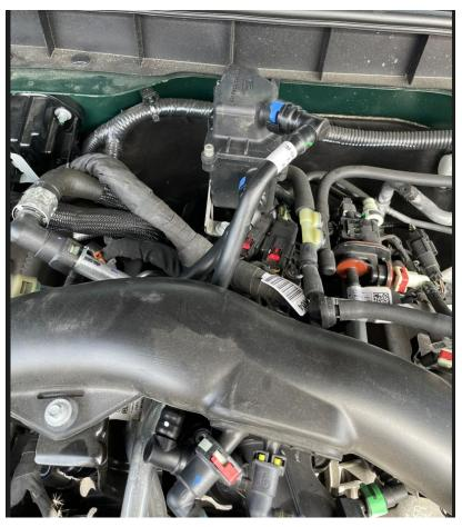
Install the oil separator on the bracket and install the RH inlet and outlet PCV tubes according to this illustration. Inlet is from the camcover to the lower spigot on the oil separator.
