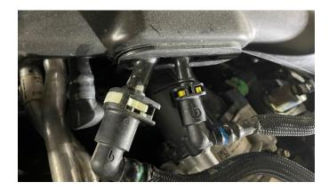
Starting with the RH side, remove the PCV tube by releasing the tang on the connectors and pulling up, removing the connector from its spigot.
