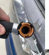
On the LH side, start by removing the tamper-proof PCV connectors. The orange inner retainer tangs will break during removal, this is normal.
