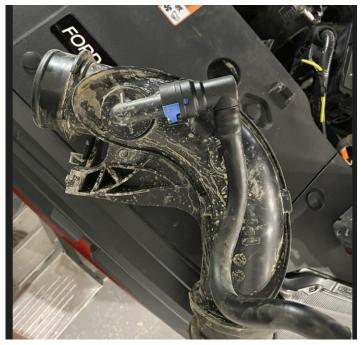
Remove PCV tube by prying loose from the spigot. The orange tangs will break, which is normal. Install new LH outlet PCV tube as shown and reinstall turbo inlet tube, torquing bolt into cyl head to 10Nm (88lbin).
