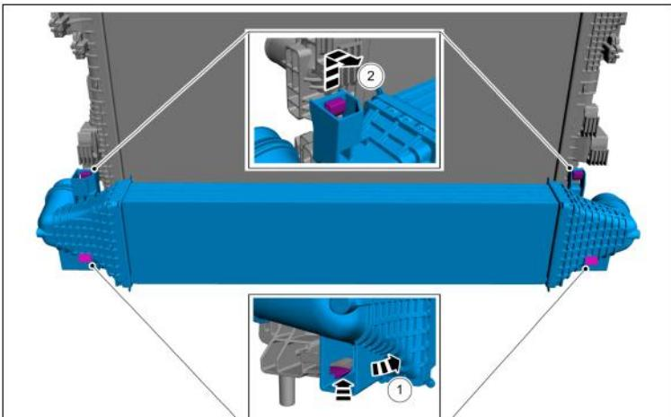
16) Unhook intercooler assembly from radiator tabs on both ends, then remove from vehicle.
