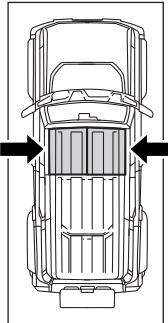
HARD TOP: Remove roof panels on both sides.
