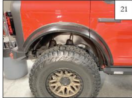
Close door and apply pressure to flare while tightening (4) screws. Open door and tighten last screw.
