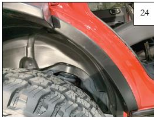
To install cover piece, remove tape liner from back of cover. Open door and align in place to cover exposed holes. Press firmly on to ensure proper adhesion.
