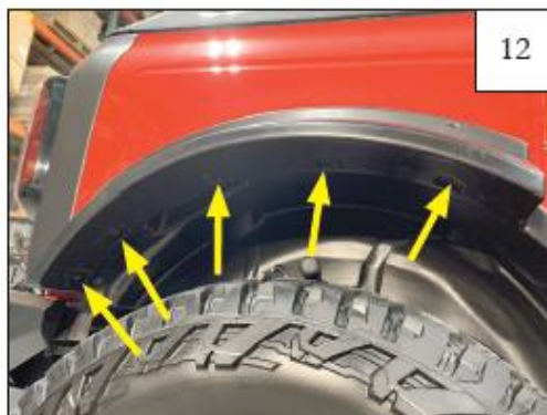
12 NOTE: Ensure that edge trim is seated correctly before proceeding. Press flares firmly onto the vehicle and install and fully tighten (5) SW1-0058 screws.
