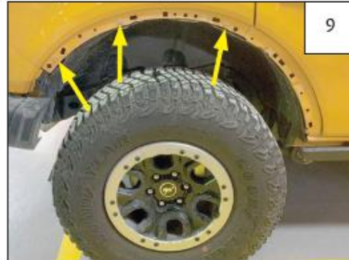
9 Remove (3) factory body bolts and retain.
