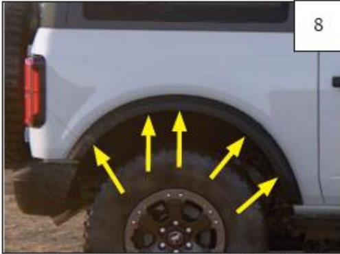
8 Twist (5) quarter turn fasteners. Firmly pull on flare to remove.
