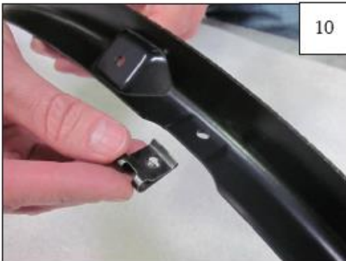
10 Verify presence of U-clip on inner brackets.
