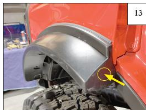
13 Use (1) SW1-0058 screw on end of flare.
