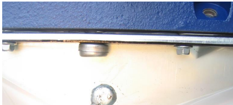
Oil pan seal location – one on each side of the oil pan
